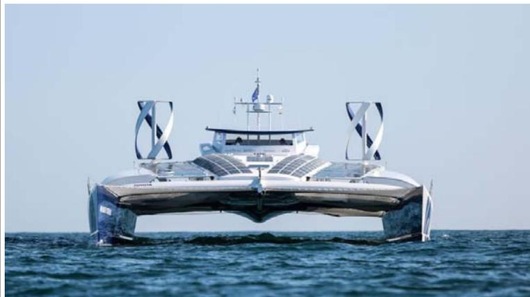
Toyota is sponsoring the world's first autonomous hydrogen-powered ship on a six-year world tour. The specially adapted race boat, Energy Observer, uses solar, wind and wave-generated power – as well as carbon-free hydrogen generated from seawater.
